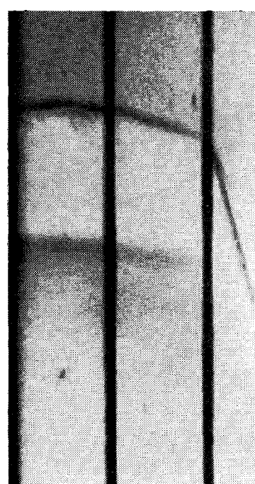
Fig. 2 Schlieren photographs of a detonation wave in a 50% hydrogen-50% oxygen mixture with a helium boundary.
