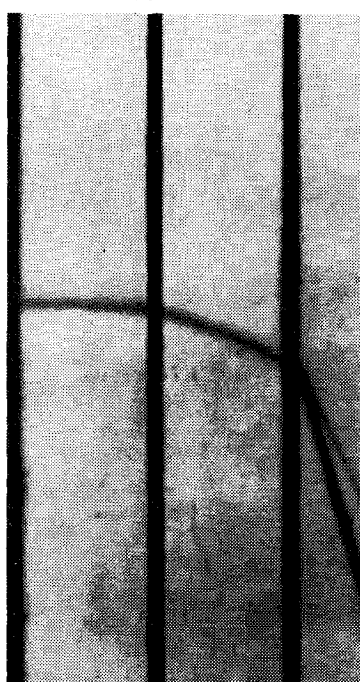
Fig. 2 Schlieren photographs of a detonation wave in a 50% hydrogen-50% oxygen mixture with a helium boundary.
