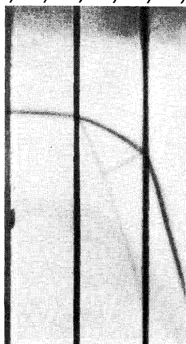
Fig. 2 Schlieren photographs of a detonation wave in a 50% hydrogen-50% oxygen mixture with a helium boundary.
